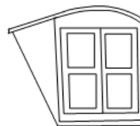
Figure 6.3: Potentially good dormer roof designs include gabled, hipped and low arched roofs.
