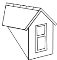
Figure 6.3: Potentially good dormer roof designs include gabled, hipped and low arched roofs.
