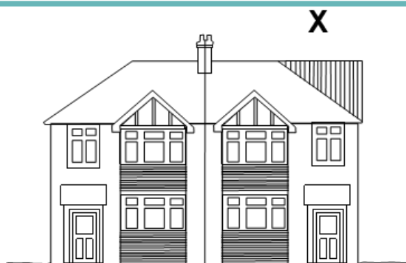
Figure 7.1: The hip to gable extension here results in a negative imbalance to the symmetry of the pair of semi-detached dwellings.
