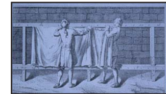
Cloth being hung to dry on a tenter frame (from Diderot's Encyclopaedia)
