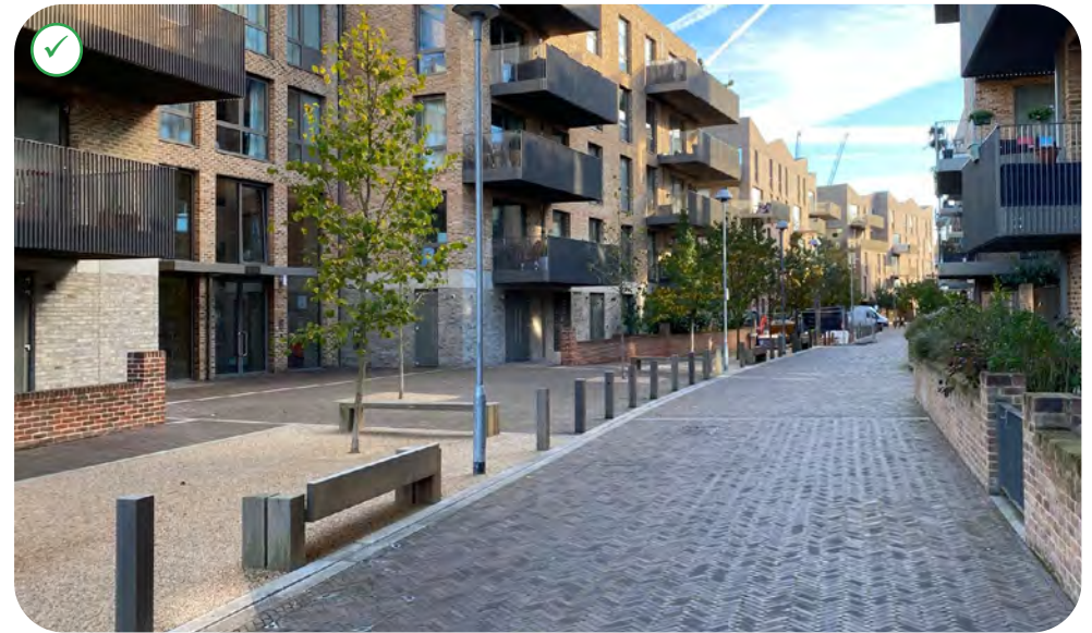
A height to width ratio of 1:1 results in good daylight access whilst still enclosing the street, Brentford Lock, London.
